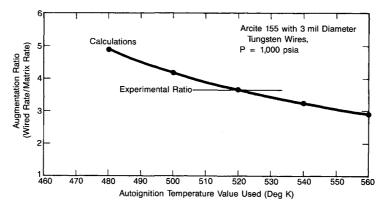
Fig. 2 Sensitivity of calculated wired propellant burning rate to input autoignition temperature.
