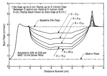
Fig. 7 Effect of ramp changes in gap width on strand burning rate vs distance burned.
