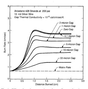
Fig. 6 Effect of gap between wire and propellant on burning rate vs distance burned.
