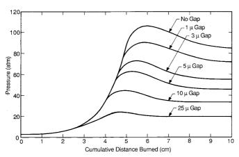
Fig. 8 Baseline motor test case—various gap widths.
