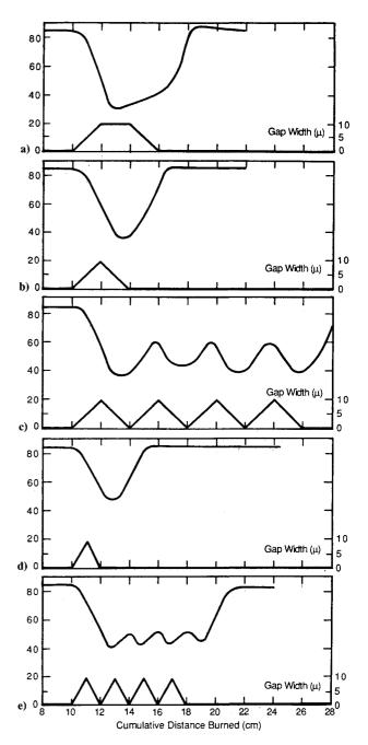
Fig. 9 Pressure (atm) vs cumulative distance burned for various gapwidth schedules.
