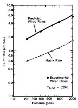
Fig. 4 Arcite 155 with 3-mil-diam tungsten wires.
