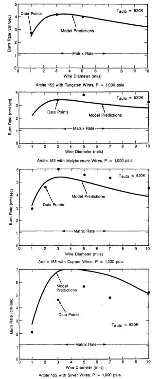
Fig. 3 Predicted and observed effects of various wires on burning rate.
