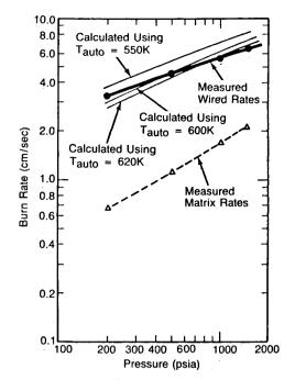
Fig. 5 Arcadene 426 with 10-mil-diam silver wires.
