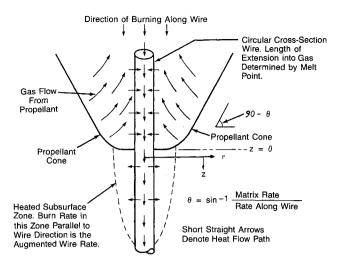
Fig. 1 Schematic of wired propellant combustion.
